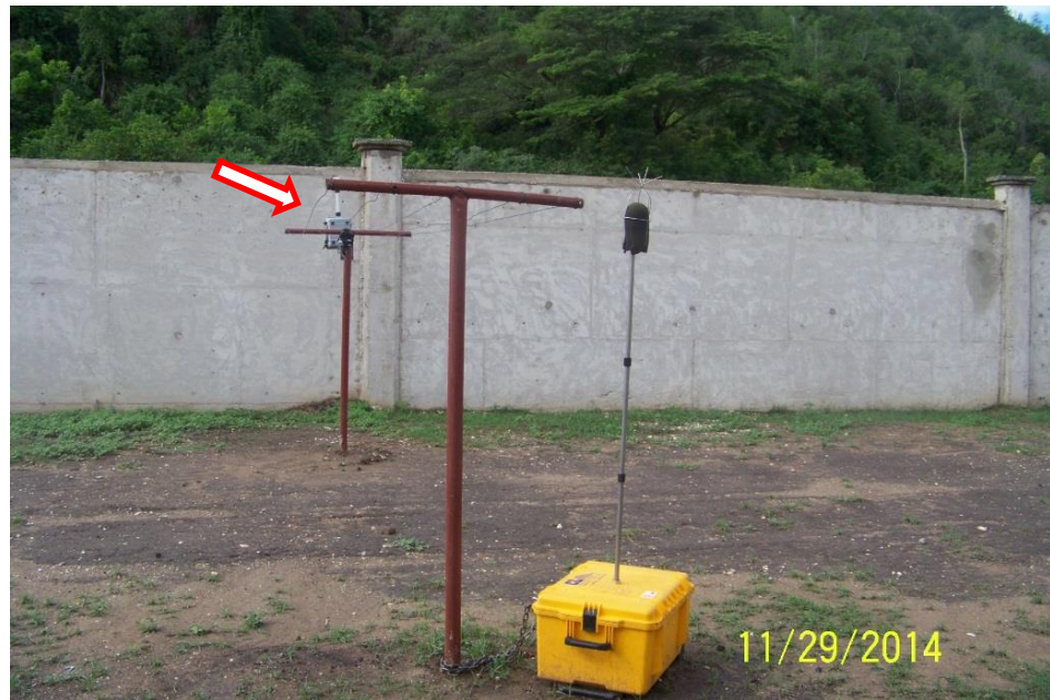
Plate 7 Photo showing noise meter at Station N1 (foreground) and particulates pump in the background (P1)
